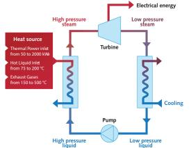
steam which will be expanded into the turbine to produce electricity (from 5 to 100 kWe). The residual heat is then evacuated through the second exchanger connected to a cooling system.
