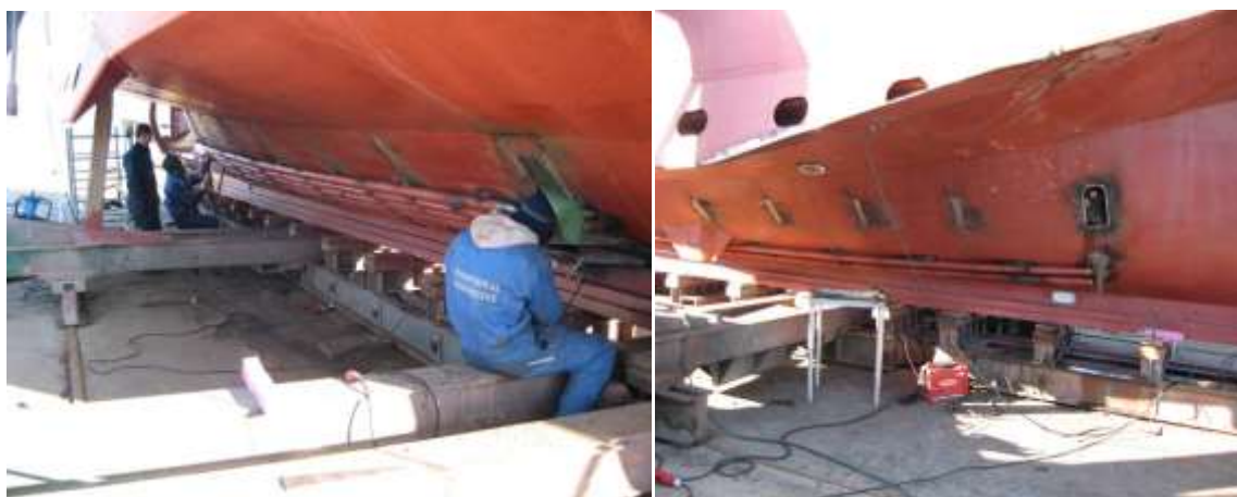
Figure 31. Modifying position of the cooling system efficiency of the propeller increase.
