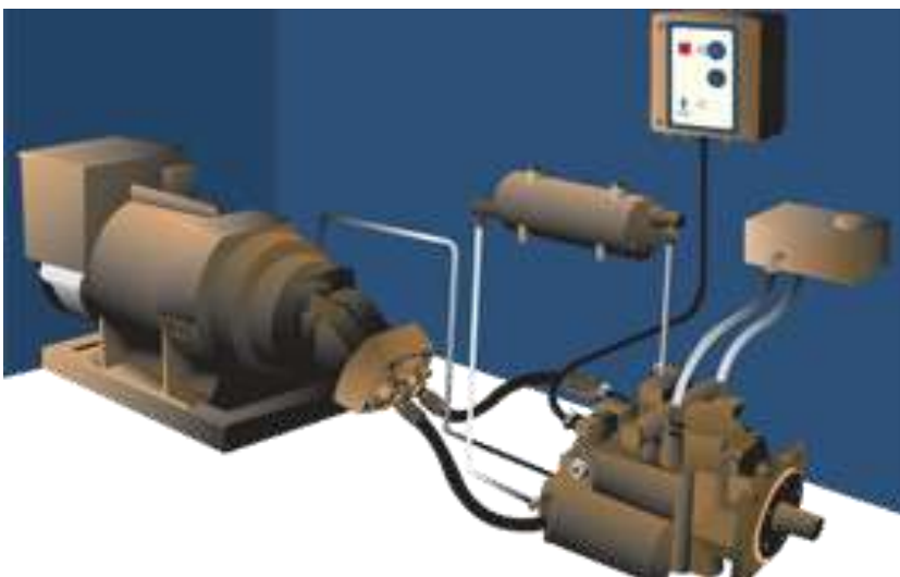
Figure 17. GENERGI system; on the left the main engine, on the right the hydraulic pump connected to a distribution header. On the top the electronic system control the operating point of the pump on the basis of the hydraulic power request
