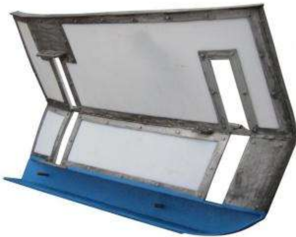
Figure 3. AR otter board with polyethylene.
