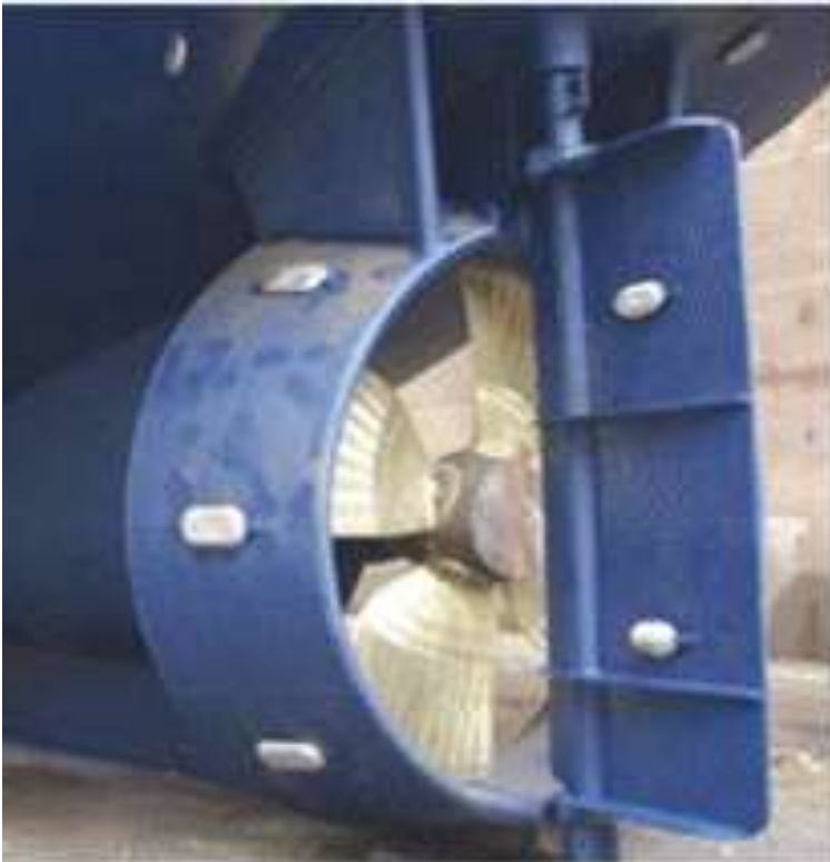
Figure 51. Ducted propeller with Kort nozzle
