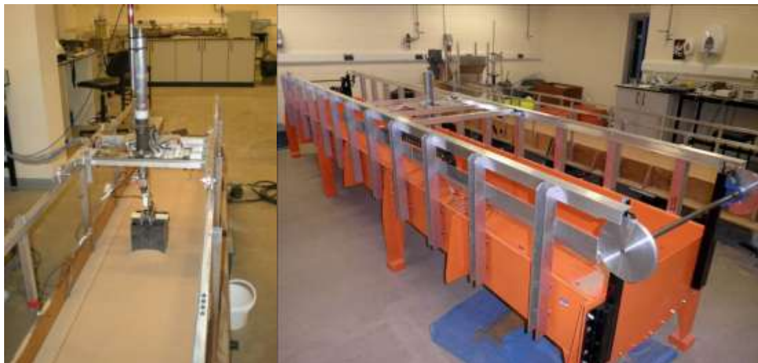
Figure 46. The Aberdeen University's geotechnical sand channels. The old one and the new one under construction.
