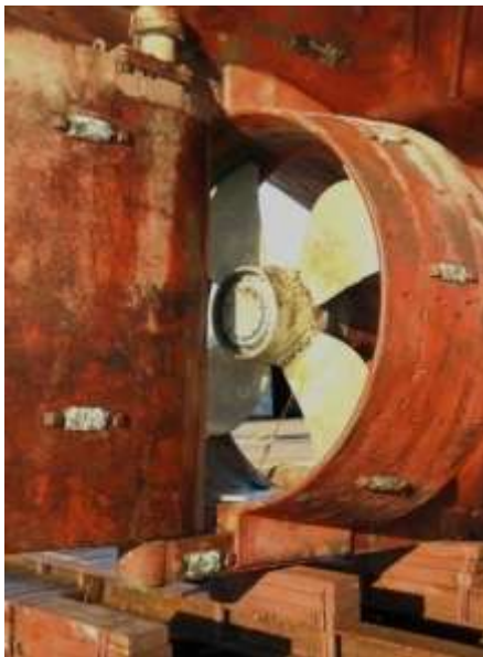
Figure 19. Propeller and propeller nozzle before and after change
