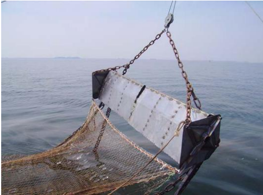
Fig. 42. Wing-shaped beam trawl – prototype 2 ('zweefkor') with runners in front (Bult, 2007)
