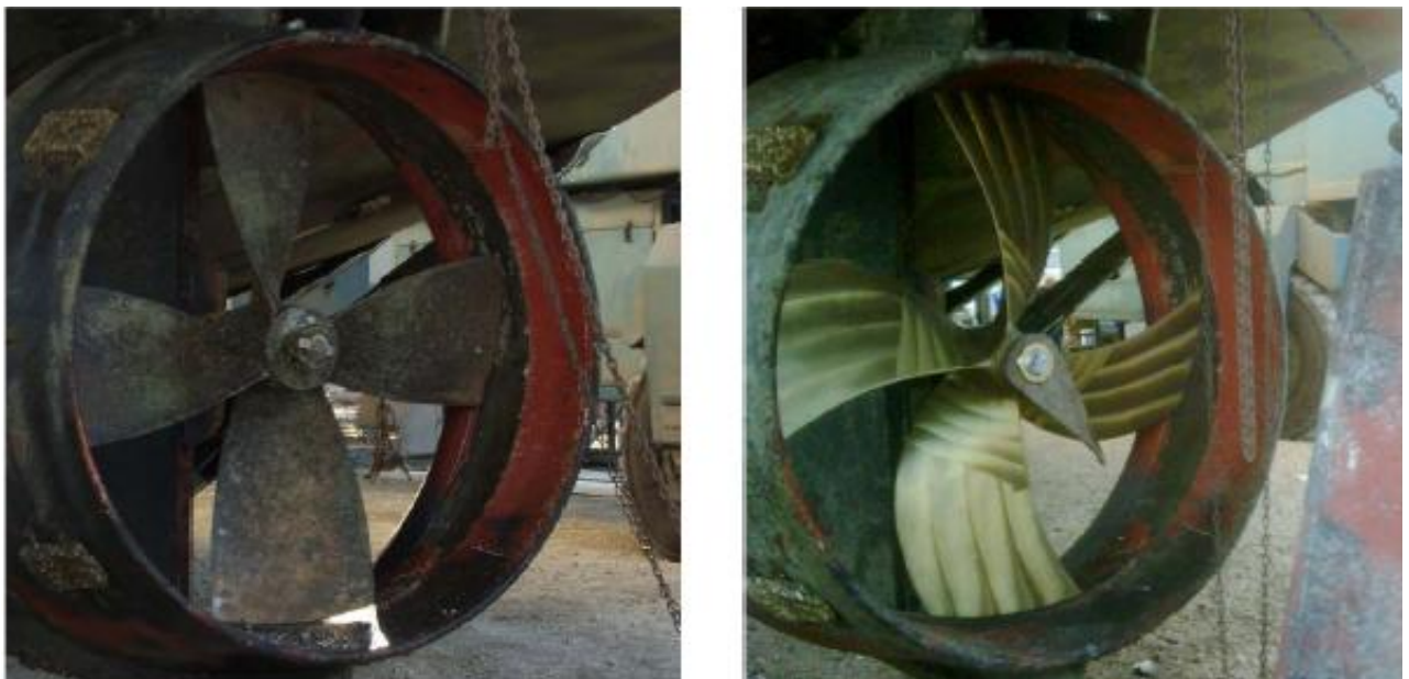
Fig. 18. Traditional Kaplan-style propeller and rice skewed wheel.
