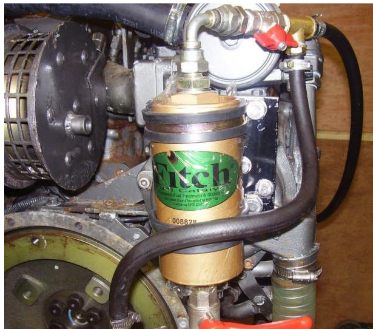
Fig. 50. Fitch system applied to a diesel engine
