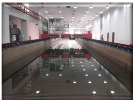
Towing tank for measuring the trawl and door performance.
