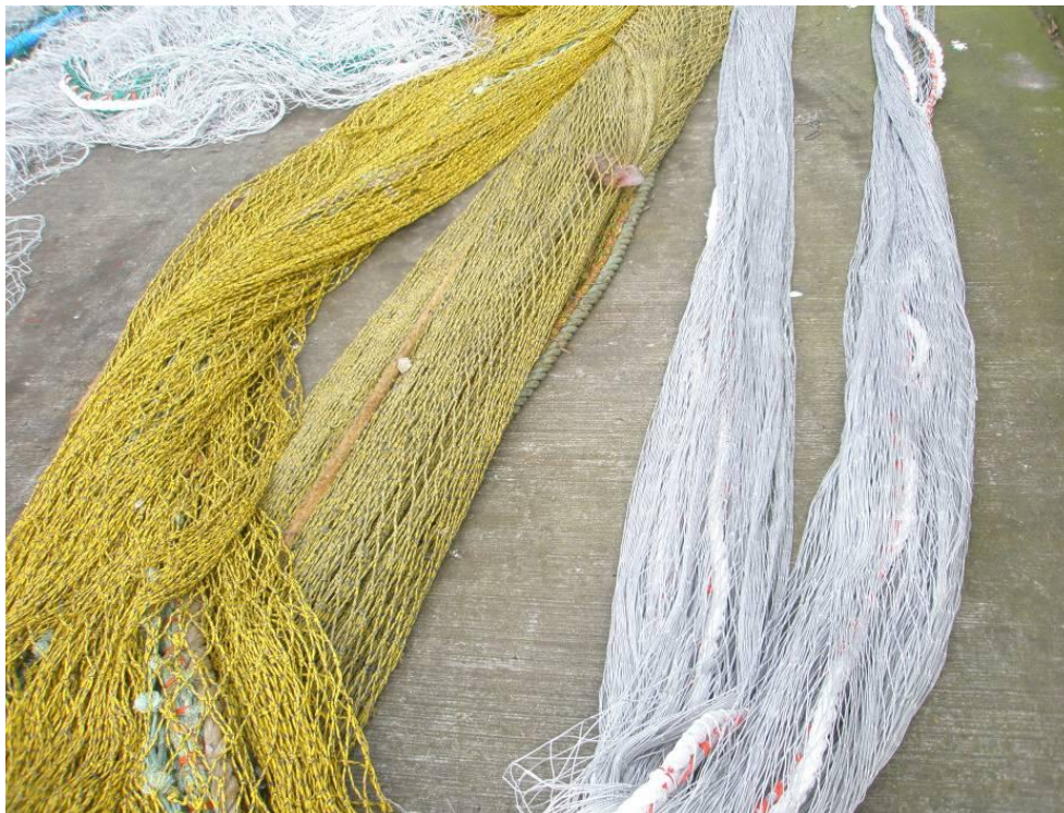
Fig. 47. Bellies of both trawls on the pier. On the left is the original net in 4.0 mm polyethylene netting whereas on the right is the 2.0 mm ultracross dyneema net.
