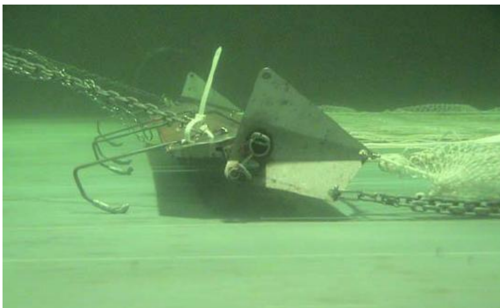
Fig. 41. Wing-shaped beam trawl – prototype 1 with runner directed aft wards (Bult, 2007)
