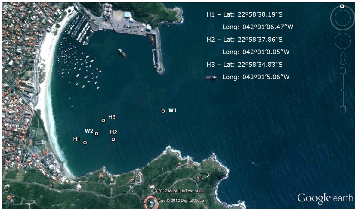
Figure 2 - Image of the place where the experiment will be conducted. H's mark the position of the hydrophones, and W's indicate the wavemeters.
