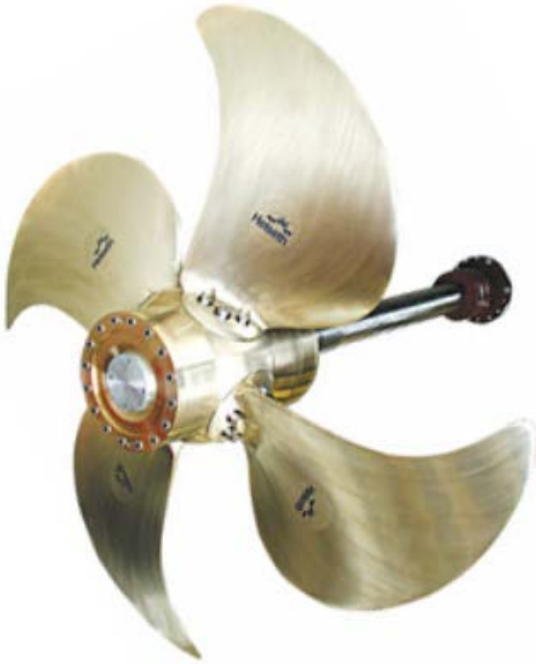
Figure 12. Controllable pitch propeller. The hub contains the hydraulic pitch control gear. One of the major advantages in using a CPP is the opportunity of substitute one propeller blade when it is damaged, instead of repairing it or changing the propeller.
