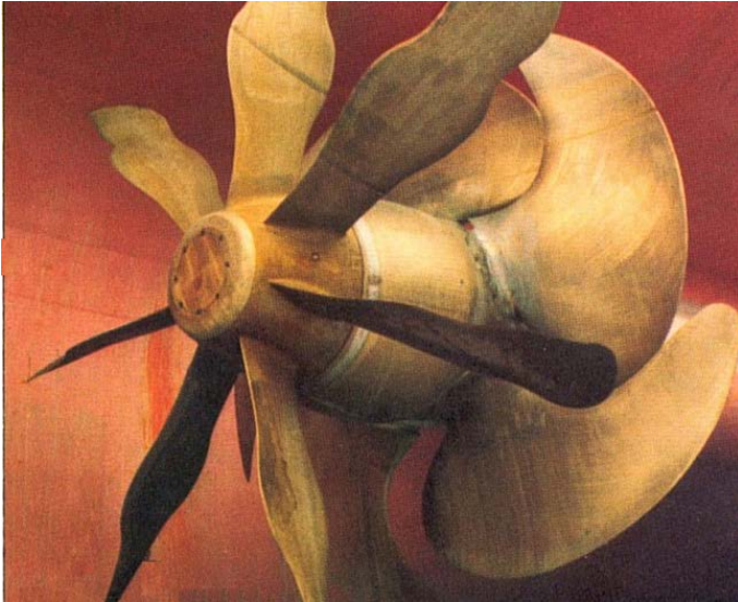
Figure 25. Greem wheel applied to a controllible pitch propeller. The Greem wheel is a free running propeller which operates as a stator, increasing propeller counter pressure thus the propeller efficiency.
